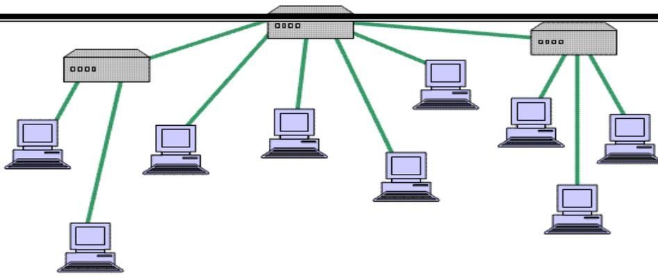
These condary hub maybe active or passive. A passive hub means it just precedes a physical connection only.
